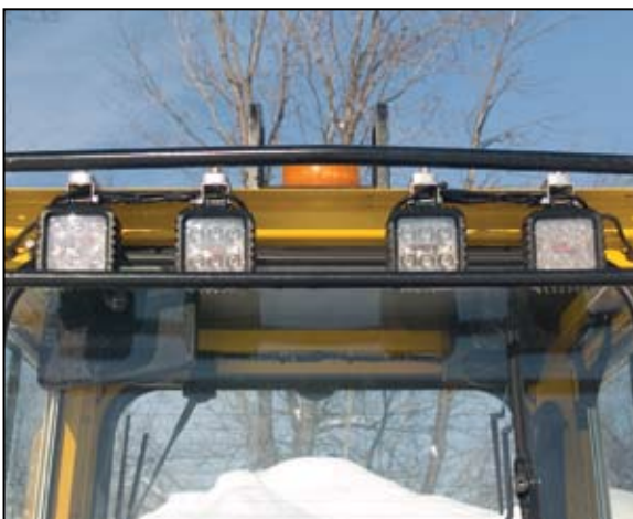
LED Work Lights do not reflect the snow like it's halogen counterparts making snowplowing easier.
