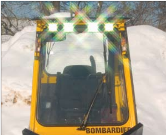
Four bright white 1000 Lumen LED Work Lights mounted the front of a Bombardier snow plow.
