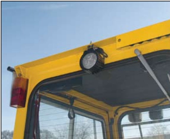
Work light shown mounted to the upper rear window of a Bombardier sidewalk snowplow.
