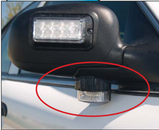
Designed to mount under the mirror on all types of vehicles or can be surface mounted to any flat area.
