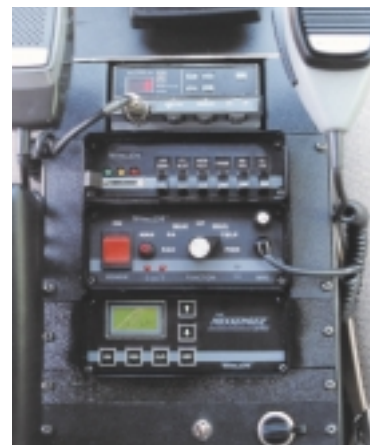
Typical police car multi-unit console with a Whelen 295HFS A1 and a PCCS9R included.
